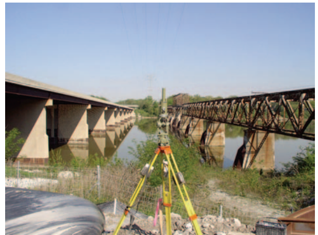
Gyroscope used to survey beneath the Maumee River connecting east river bank to west river bank.
